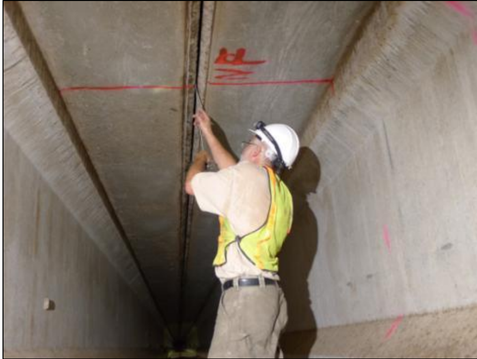
Figure 2.2. The width and depth of each gap segment at the IH 35 bridges over the Lampasas River and Salado Creek in Bell County, Texas, were measured to the nearest centimeter in order to calculate the volume of the available habitat.
