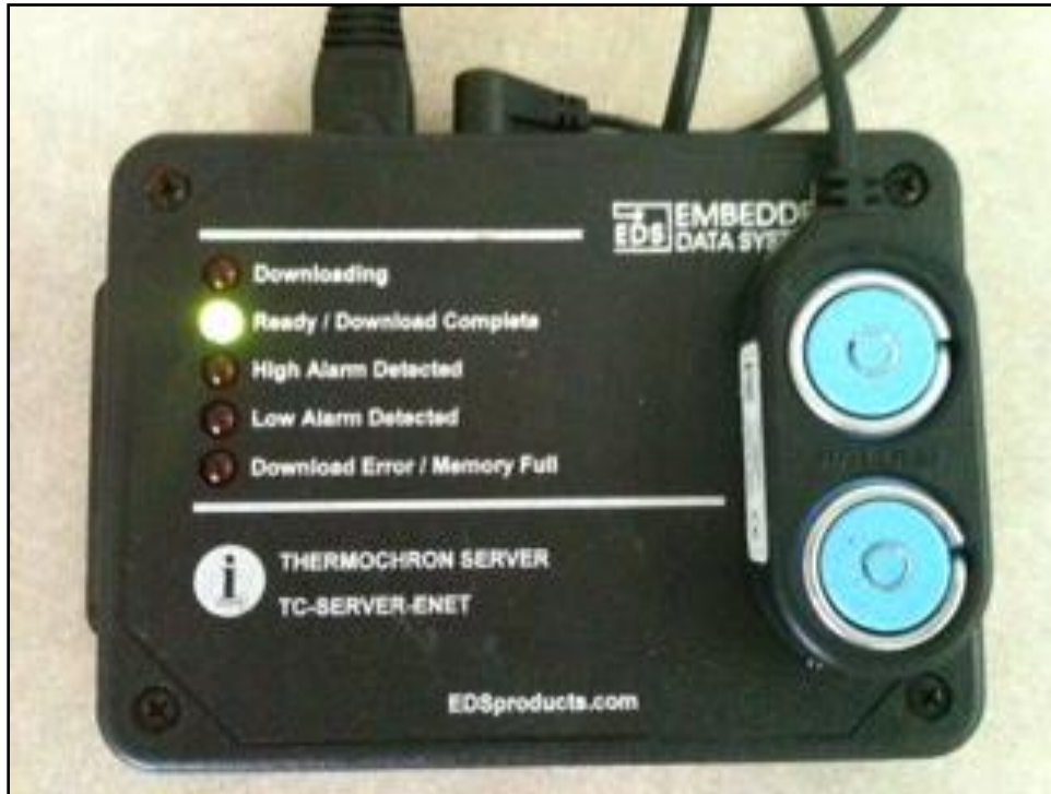
Figure 2.5. ThermoChron Server from Embedded Data Systems used to download iButton data.
